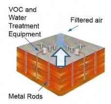
illustration). An engineered cover with a dedicated vapor recovery system was installed over the treatment areas to ensure vapors do not escape to the atmosphere from the soil surface.
